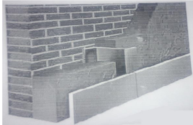
Figure 1.4. Constructive solution for the facade of the ventilated air gap of the PAROC system.
